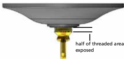
Drawing 2 Canopy Adjustment
