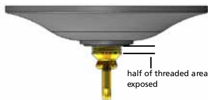
Drawing 2 Canopy Adjustment
