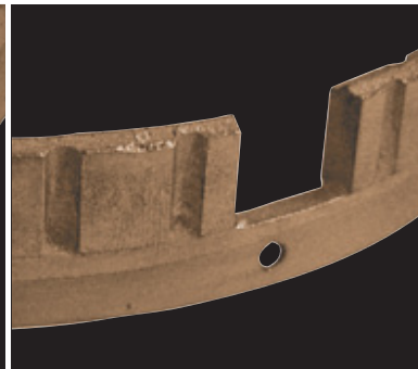
Solder capillaries improve attachment.
