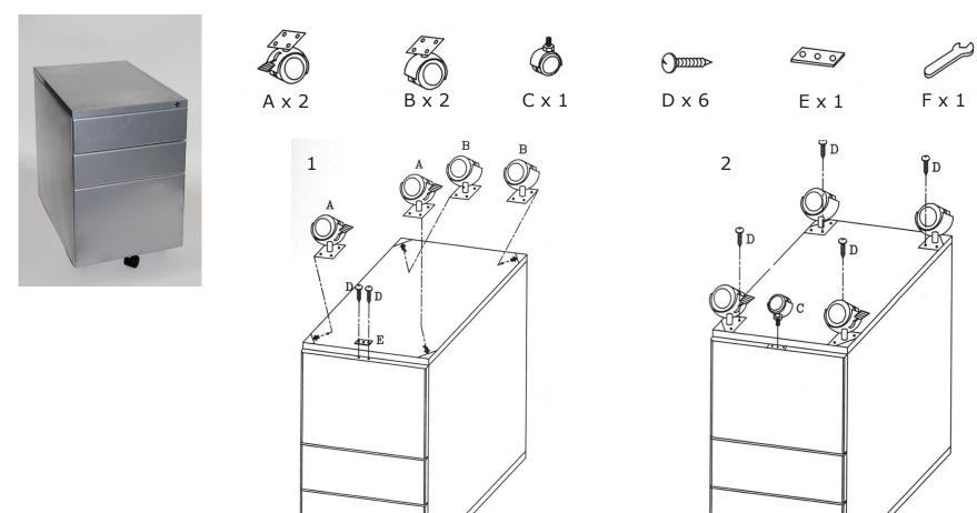
During assembly, hand tighten screws only. When all screws are in place, then tighten completely.
