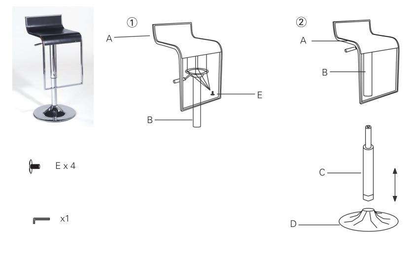
During assembly, hand tighten screws only. When all screws are in place, then tighten completely.
