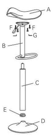
During assembly, hand tighten screws only. When all screws are in place, then tighten completely.
