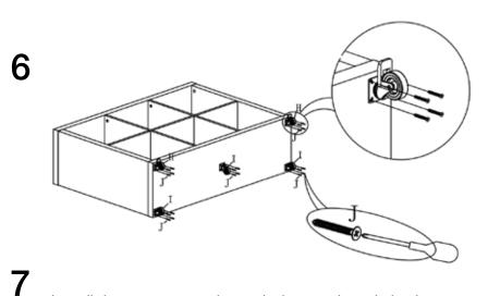
Install the casters as shown below and apply brakes on the casters when the shelf is at the desired location.
