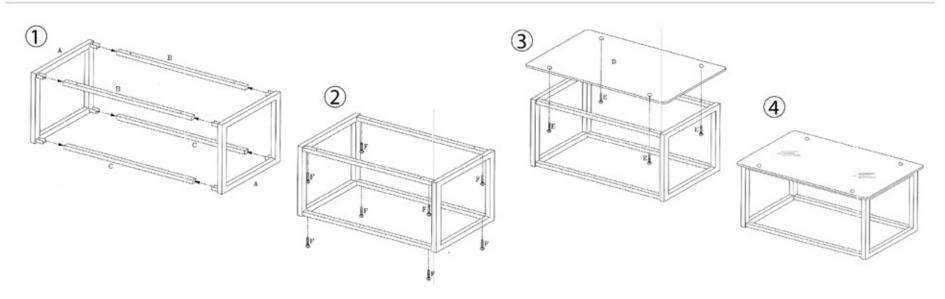
During assembly, hand tighten screws only. When all screws are in place, then tighten completely.
