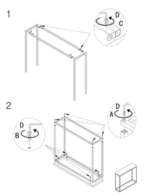
During assembly, hand tighten screws only. When all screws are in place, then tighten completely.
