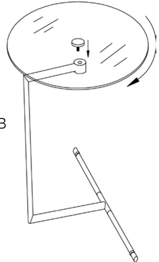
During assembly, hand tighten screws only. When all screws are in place, then tighten completely.
