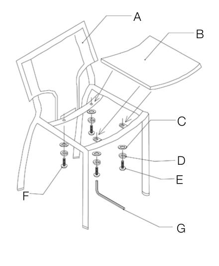
During assembly, hand tighten screws only. When all screws are in place, then tighten completely.
