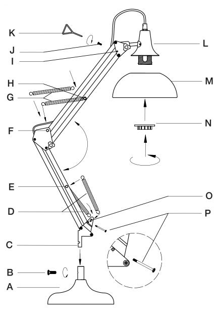
During assembly, hand tighten screws only. When all screws are in place, then tighten completely.
