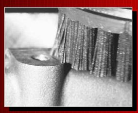
Disc brushes are ideal for deburring flat surfaces after face milling. On such parts, all burred edges are on the same plane and are easily deburred.
