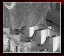
Large diameter wheel brushes are used to focus significant deburring energy on targeted edges. The steel inserts in this aluminum engine component have a severe burr condition requiring the aggression of wheel brushes.
