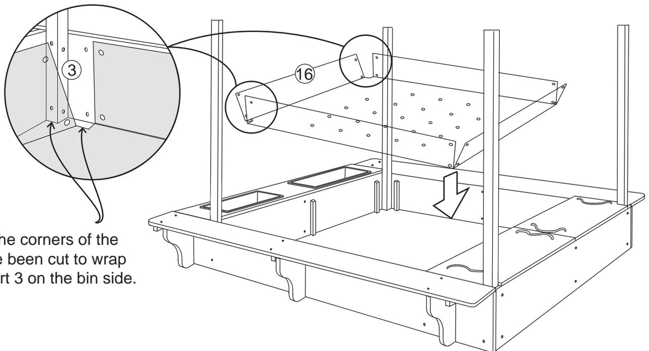
Two of the corners of the liner have been cut to wrap around part 3 on the bin side.
