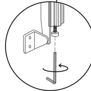
Check periodically to make sure the lid is not falling shut. If the lid is starting to slowly fall shut, adjust the braking tension (set screw) with a 4mm hex key until the lid will remain open when you let go of it.
