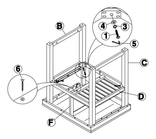
Attach bottom frame (E) to right side frame (B) and left side frame (C) with bolts (2) and washers (3) and (4). Tighten with Allen key (5).
