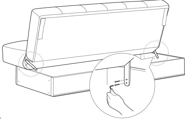
Screw in four threaded rods into pre-drilled holes on the inner side of armrest by hand until about half of the thread is exposed. Repeat step for other armrest.
