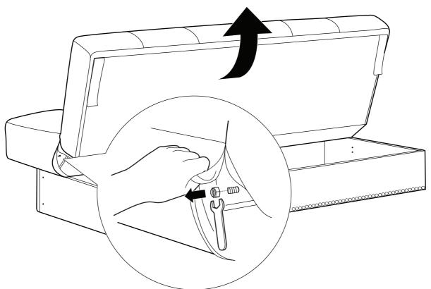
3 Connect metal bar into exposed fix threaded rod as shown below and secure with nut (B) using the spanner. Do not tighten completely yet.
