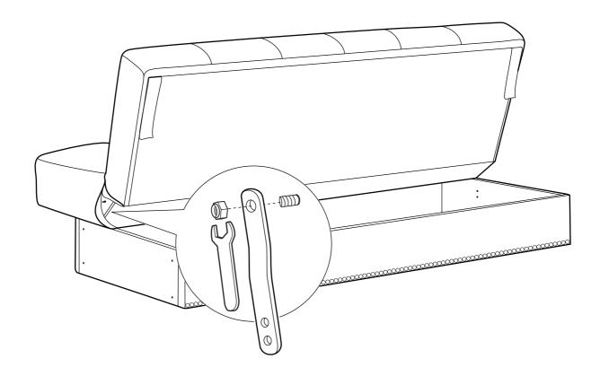
4 Carefully align metal bar onto the pre-drilled holes inside storage body unit as shown. Secure two bolts for each metal bar into pre-drilled holes using provided Allen key. Completely tighten all bolts and nuts.
