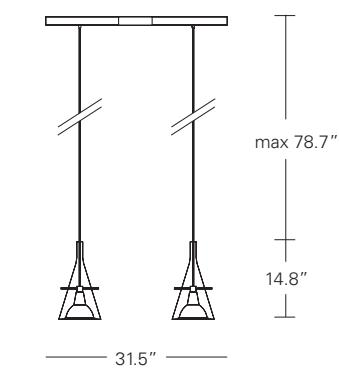
**Flûte 3** is provided with three diffusers mounted on a raceway having a 19.7" distance between centres. Borosilicate transparent glass structure. Polished chrome-plated aluminium reflector. Transparent feeding cord.
