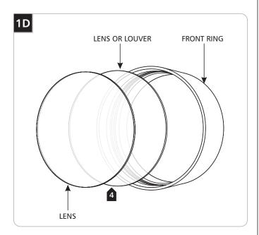
4 Place one or at most two lenses and/or louver into the front ring.
