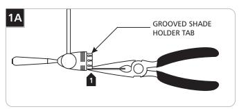
1 If the Scavo accessory fits tight onto the fixture, then carefully bend the grooved shade holder tabs in slightly with the needlenose pliers. If it fits loose, then carefully bend the grooved shade holder tabs out slightly with the needlenose pliers.
