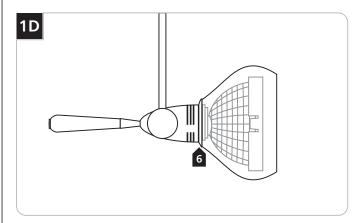
6 Hold the lamp against the glass with the thumb and push the lamp pins completely into the socket holes; simultaneously push the Scavo accessory metal ring onto the grooved shade holder.
