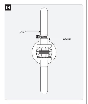
Use **MAX** 120 Volt, **60** Watt Type T10 Medium Base Lamp, For Each Socket.
