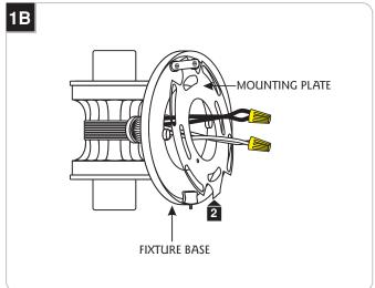
**2** Pull out the mounting plate from the fixture base.
