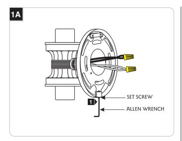
With the provided Allen wrench unscrew (**Do Not Remove**) the set screw on the bottom of the fixture base.
