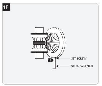
Line up the fixture on the wall and then secure it to the mounting plate by tightening the set screw at the base of the fixture.
