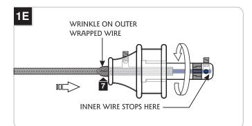
Keep pushing the coaxial cable into the connector while rotating the connector to ease feeding the inner wire into the tip of the connector. The outer wrapped wire will start wrinkling while being inserted another 1/2" into the connector.
