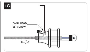
**10** Tighten the #6-32 oval head set screw on the conical connector firmly.
