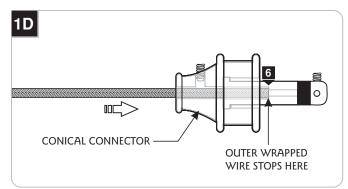
Feed and push the coaxial cable into the conical connector.
