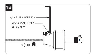
Back out (Do Not Remove) the #6-32 oval head set screw on the conical connector with the provided 1/16 Allen wrench.
