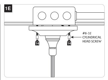
Place all wires and wire nut connections properly into the electrical box and mount the canopy to the electrical box with the provided two #8-32 cylindrical head screws.
