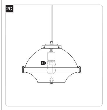
4 Push the lamp shield onto the spring clips.
