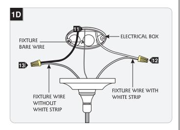
**NOTE:** Use the provided universal round crossbar when the canopy holes do not line up with the electrical box holes.
