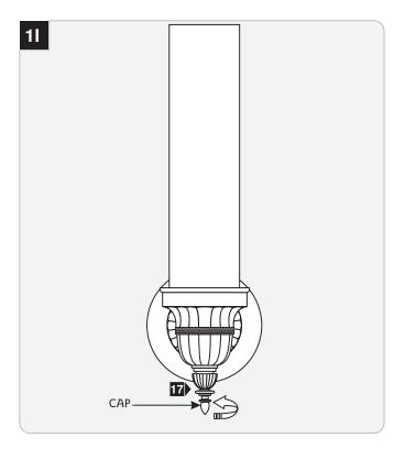
**17** Use the cap to turn the fixture on/off by rotating it clockwise.
