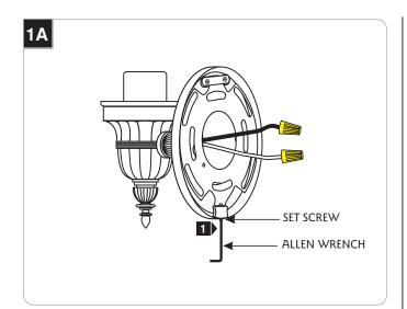
With the Allen wrench provided, back out (**Do Not Remove**) the set screw at the base of the sconce.
