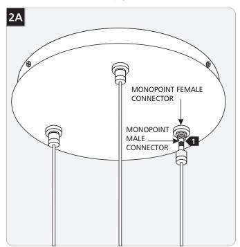
Screw the fixture MonoPoint male connectors into the canopy female connectors.
