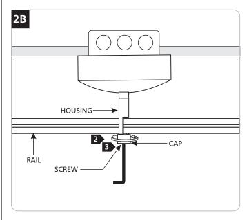
2 Replace and tighten the cap to the housing.
