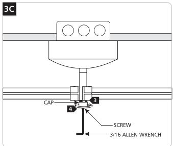
Replace and tighten the cap to the housing.
