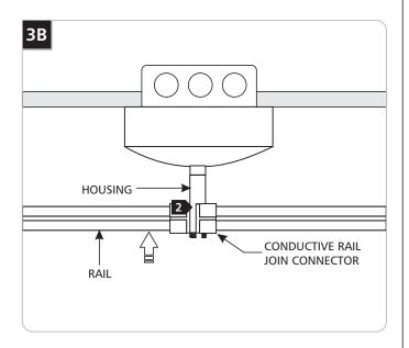
2 Push the conductive rail join connector into the housing.
