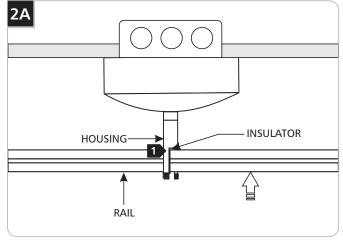
Push the rail into the housing so that the rail fits in the middle of the insulator.
