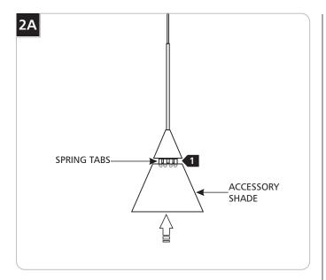
1 Push the accessory shade all the way onto the spring tabs.
