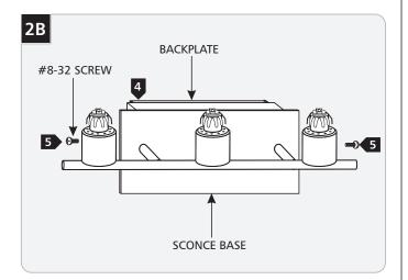
4 Place the sconce base onto the backplate and align the holes.
