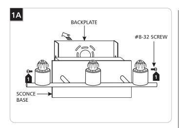
1 Remove the two #8-32 screws on the backplate with a Phillips head screwdriver.
