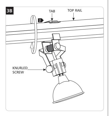
2 Rotate the Axis until the tab on the spring snaps onto the top rail.
