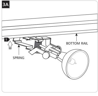
Connect the Axis by placing the open part of the springs onto the bottom rail.
