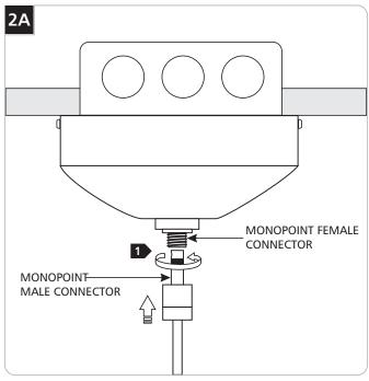
Push the fixture MonoPoint male connector all the way into the surface canopy MonoPoint female connector. Tighten the male connector.
