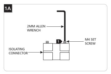
Back out (DO NOT REMOVE) the two M4 set screws with 2MM Allen wrench to clear the connector open ends.
