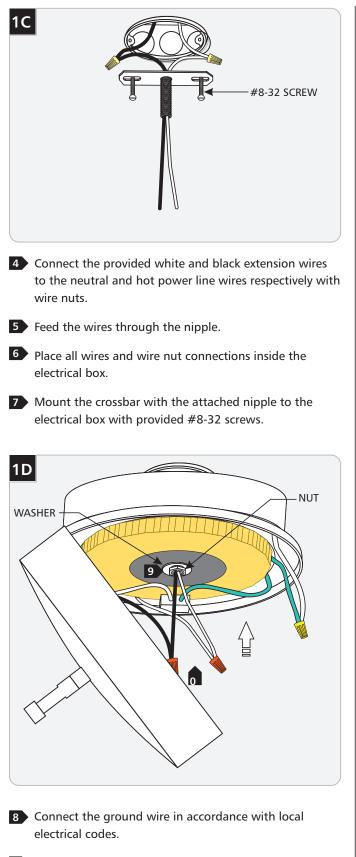
9 Slip the transformer housing and the washer onto the nipple and tighten the inside nut to secure the transformer housing.
