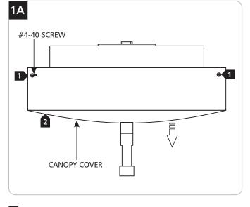
On the side of the transformer canopy cover, remove the #4-40 screws with a Phillips head screwdriver.
