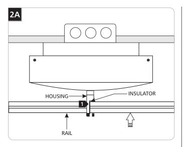
1 Push the rail into the housing so that the rail fits in the middle of the insulator.
