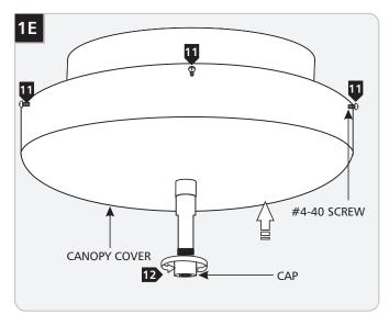
**1** Replace the canopy cover onto the transformer housing. Line up the canopy cover holes with the transformer housing holes. Replace and tighten the #4-40 screws.
