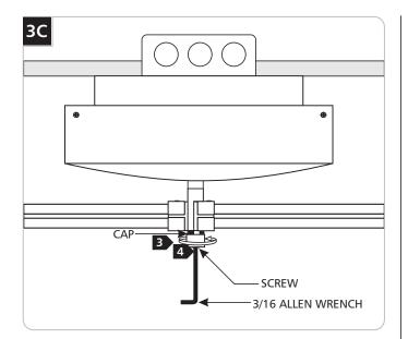
3 Replace and tighten the cap to the housing.
