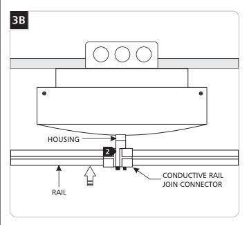
2 Push the conductive rail join connector into the housing.
