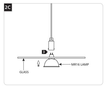
Use MAX 50 Watt, MR16 Front Cover Halogen Lamp.
