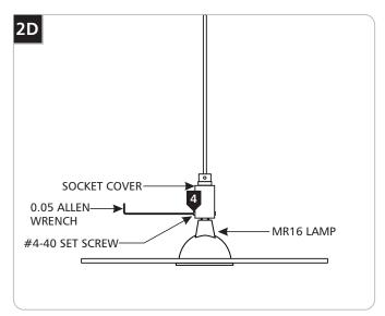
4 Hold the glass in place and tighten the two#4-40 set screws on the socket cover with the 0.05 Allen wrench.
