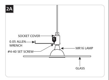
Hold the glass with one hand and loosen the two #4-40 set screws on socket cover with the 0.05 Allen wrench.
