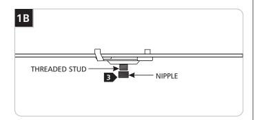
3 Screw the threaded nipple onto the T-bar threaded stud.
