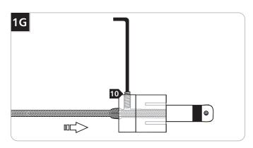
Tighten the #6-32 oval head set screw on the cylindrical connector firmly.
