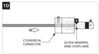
6 Feed and push the coaxial cable into the cylindrical connector. The coaxial cable will come to a stop point after being inserted 3/4" into the cylindrical connector.
