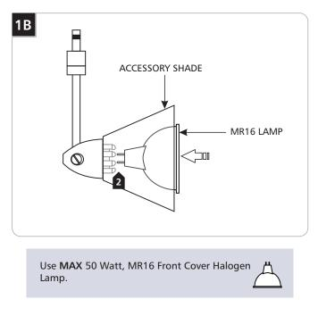
2 Line up the lamp pins with the socket holes. Insert the MR16 lamp pins all the way into the socket holes.
