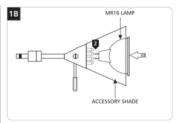
Use MAX 50 Watt, MR16 Front Cover Halogen Lamp.
