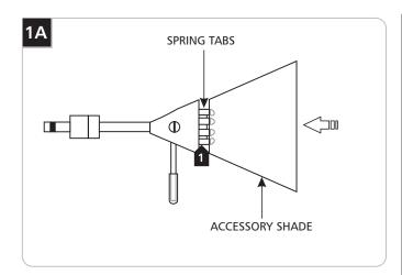
1 Push the accessory shade all the way onto the spring tabs.
