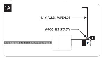
1 Back out (DO NOT REMOVE) the #6-32 set screw on tip of the connector with the provided 1/16 Allen wrench.
