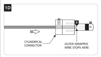
6 Feed and push the coaxial cable into the cylindrical connector. The coaxial cable will come to a stop point after being inserted 3/4" into the cylindrical connector.
