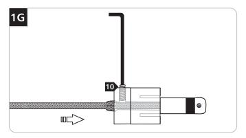
10 Tighten the #6-32 oval head set screw on the cylindrical connector firmly.
