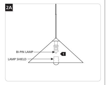
Use MAX 50 Watt, Bi-Pin Halogen Lamp.
