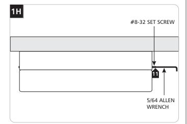
Tighten the two #8-32 set screws with the 5/64 Allen wrench.
