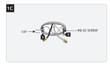
Thread (NOT COMPLETELY) the two #8-32 screws into the electrical box holes leaving 1/4" of them exposed.
