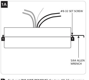
Back out (DO NOT REMOVE) the two #8-32 set screws for 1/4" with the 5/64 Allen wrench.
