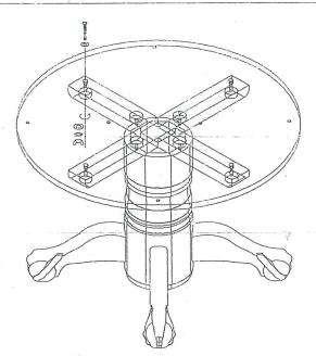
ASSEMBLE THE BASE PLATE TO THE 2 CROSS RAILS .
