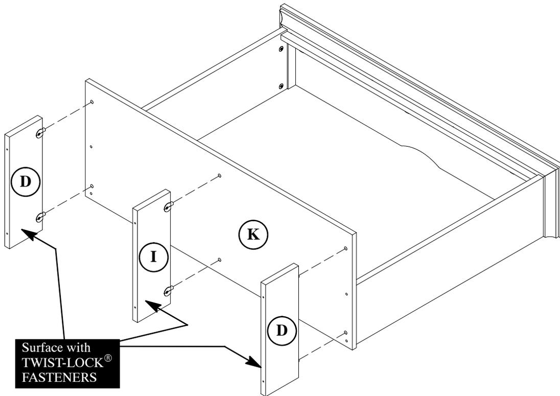
How to use the SAUDER TWIST-LOCK® FASTENER (Refer to the enlarged diagram.)
