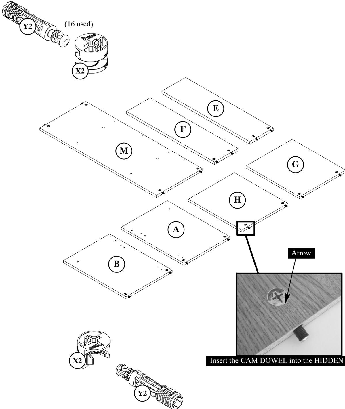
☐ Push sixteen HIDDEN CAMS (X2) into the ENDS (A, B, E, and F), UPRIGHTS (G and H) and BOTTOM (M). Then, insert the metal end of a CAM DOWEL (Y2) into each HIDDEN CAM.
