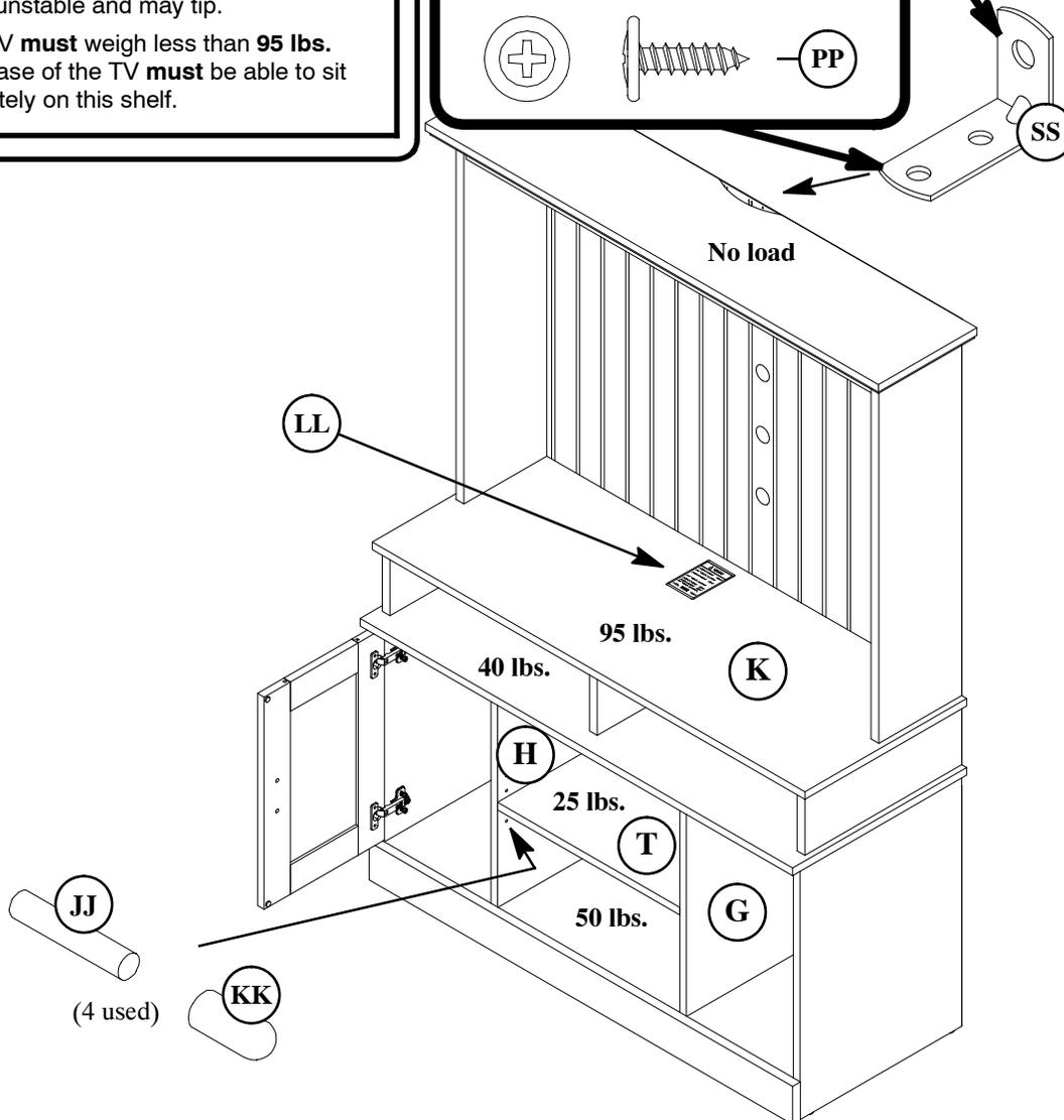
Apply the WARNING LABEL (LL) to the TOP (K). You should be able to read the label when the TV is removed from the unit. When the TV is in place, it should hide the label. Peel off the backing and apply the label as shown in the diagram.
