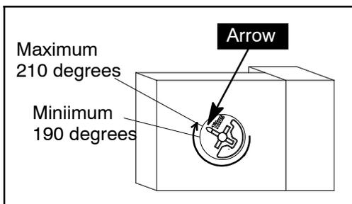
Fasten the ENDS (A and B) to the SHELF (J) and BOTTOM (M). Tighten eight HIDDEN CAMS.
