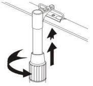
5. Rotate the locking ring clockwise to lock the upright support at its desired height setting.
