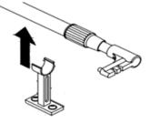
2. Insert the upright support into the socket on the center base foot.
