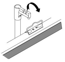
3. Rotate the locking ring clockwise to secure the upright support and remove it from the socket on the center base foot.
