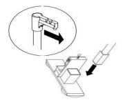
3. Hang the suspension handle of the screen from either of the notches of the upright support.
