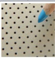
Elite's CineWhite-Perforated™ Screen Material is the answer for acoustic transparency in a tension screen. CineWhite™ material features broad light dispersion with spectral uniformity, panoramic viewing angle and true color rendition. Its 0.3mm micro-perforations create acoustic transparency by providing outstanding sound quality at dampening at 20 KHz only 2.0dB and Max. Attenuation at 20cm is 1.1db. Elite CineWhite-Perforated makes the picture sound as good as it looks.
