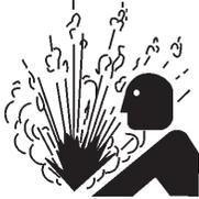
■ **NEVER** open the priming plug when pump is hot. Hot water inside could be pressurized much like the radiator of an automobile. Allow pump to cool to the touch before loosening plug. The possibility exists of scalding, resulting in severe bodily harm.
