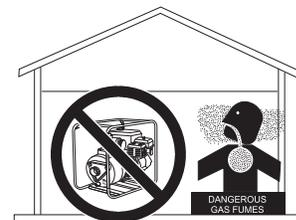
■ **ALWAYS** refuel in a well-ventilated area, away from sparks and open flames. **DO NOT** fill the fuel tank while the engine is running or hot. **DO NOT** overfill tank, since spilled fuel could ignite if it comes into contact with hot engine parts or sparks from the ignition system. Store fuel in approved containers.
