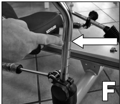
It is recommended that you first try positioning the clamp the lower knurl marks, between 1 – 10, and then if you wish for more resistance, adjust to higher knurl marks.
