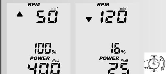
If the displayed performance cannot be achieved at a given pedal rate in non-rpm-linked mode, an upwards- or downwards-pointing arrow will be displayed.
