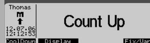
Press "CoolDown" to display a progress bar.
