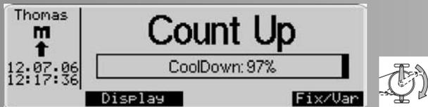
Example: When the CoolDown performance = 100% is reached, there will be 3 audible signals and the function terminates.
