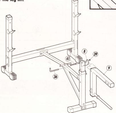
Slide the Leg Lift Crossbar (10) into either of the two holes at each end of the Leg Lift (9).
