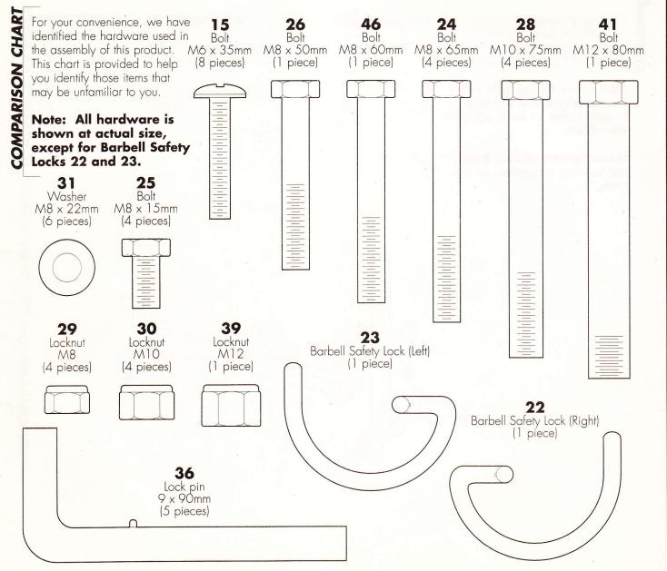
Connect the Upright Cross Bar (2) to both Upright Stanchions (1) and secure with Bolts (28), Locknuts (30), and 60mm Support Plates (40).
