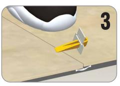
Once the mortar sets, simply kick the clips, forcing them to snap off at the specially designated break-points.
