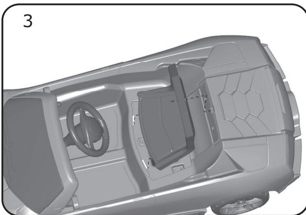
*Note: Please make sure to connect the Red Plug to the Battery Plug first before installing the seat.*
