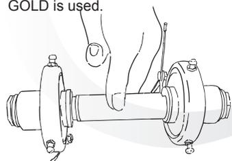
2. The GOLD axle has a reverse thread so turn anti clockwise to locate into the cassette.
