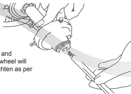
4. Check that the axle is fully located by ensuring that only the thread is visible as shown.
