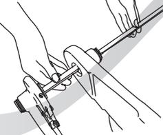
6. Ensure that Black Locknut is fully tighten and secure
