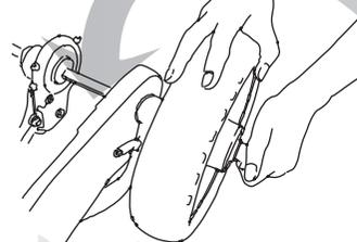
5. Thread Black Lock Nut onto axle
