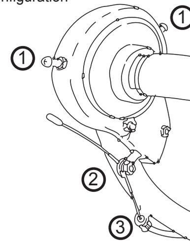
3. Fine Adjuster Feral - there are two on the front fork and it is important when adjusting the brakes that they are balanced to ensure even braking
