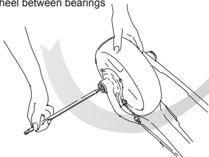
2. Insert Medium Axle through wheel bearings and wheel
