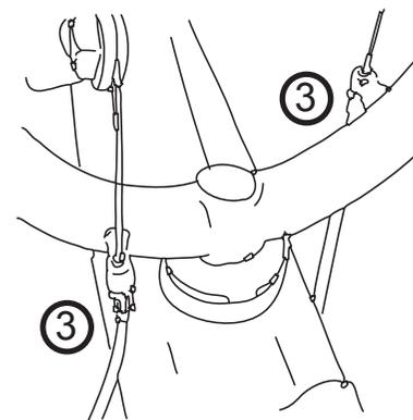
4. Cable Splitter Adjuster Feral Check that these are tighten and use to adjust the cable.
