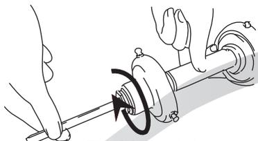
3. Using the spanner supplied hold the bearing and using the wheel turn anti clockwise until the axle is tight and secure. THIS IS VERY IMPORTANT.
