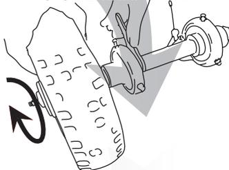
5. Insert second axle on right hand sides through bearing and locate into the cassette.
