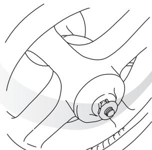
8. For both axles place the lock nut on the axle and using the spanner ensure that the nuts are fully tighten. There should be no wobble or movement sideways. Check Fig. 4
