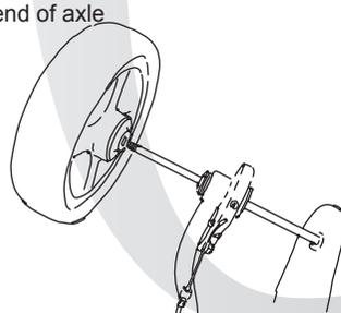
8. Thread Black Lock Nut onto axle and ensure that it is fully tighten and secure
