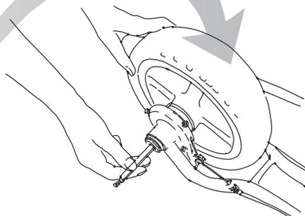
4. Thread Black Lock Nut onto axle and ensure it is fully tighten and secure
