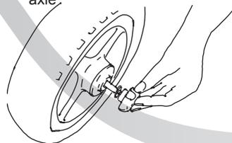
4. Place washer onto axle as shown
