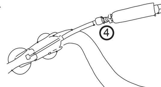
**NB.** Now that you have adjusted the band brakes, test by rolling the bike forward and apply the brake, if there is any pull to the left or right adjust the feral to achieve a balance between the two band brakes.
